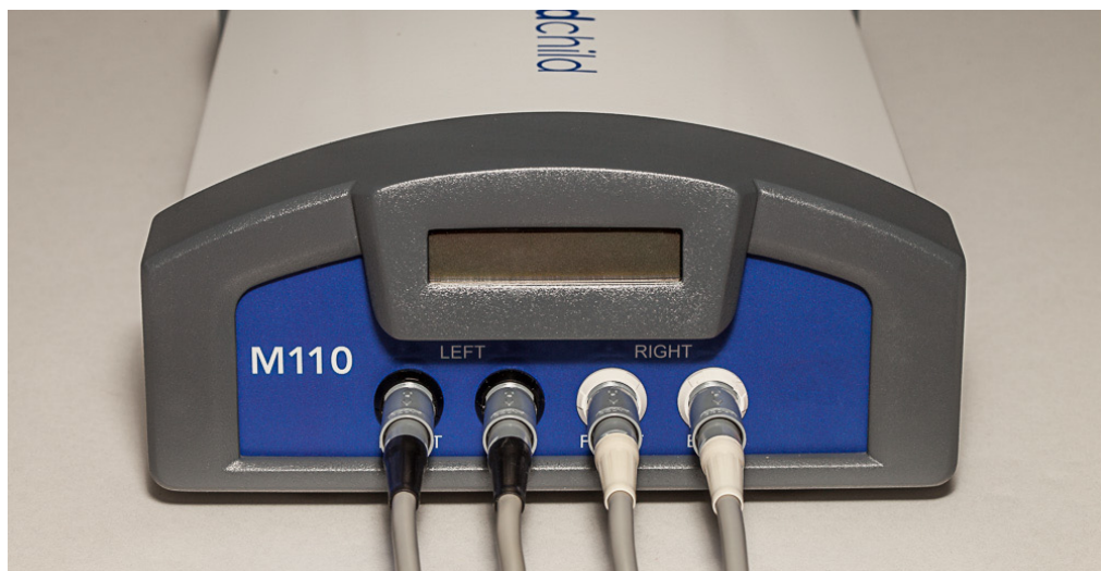
Figure 29. M110 with All Patient Cables Connected
