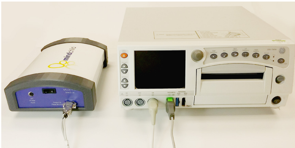
Figure 9b. M110 connected to a GE Corometrics 250 Fetal Monitor
