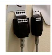
A small portion of the silver tab is visible even when it is fully inserted into the cable connector.
