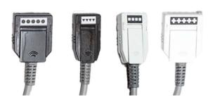
Each cable has a pattern that corresponds with its matching patch. White patterns match with right patches and black patterns match with left patches.
